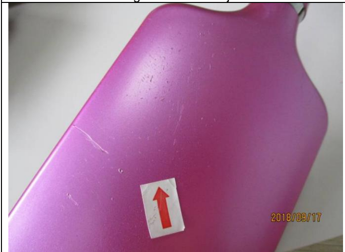
Rough surface – Major
