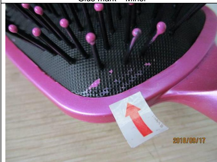
Poor finishing – Minor
