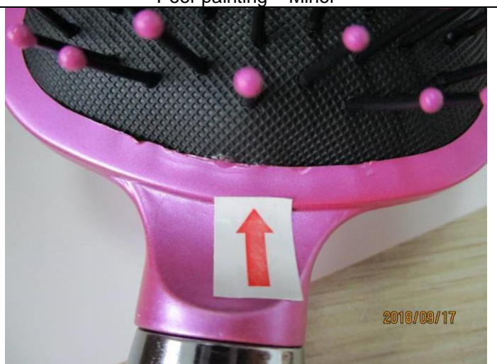
Rough edge /Rough surface – Minor
