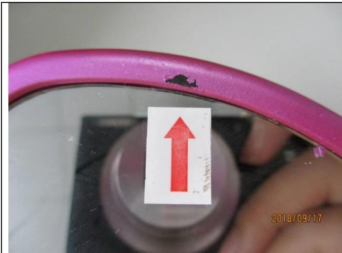
Poor painting – Major
