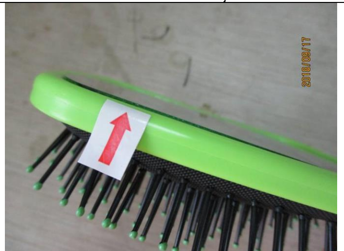
Poor assemble – Major
