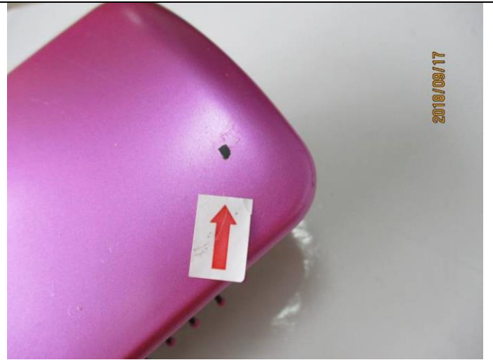
Poor painting – Major
