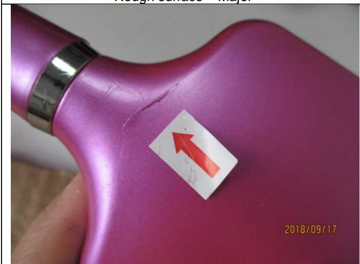
Rough surface – Minor
