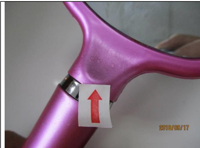
Rough edge /Rough surface – Minor
