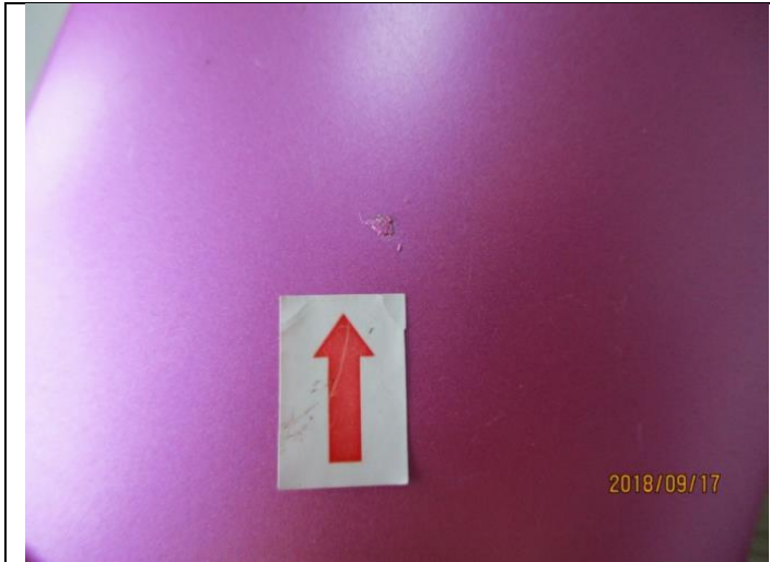
Rough surface – Minor
