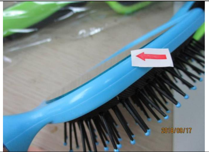
Poor assemble – Major
