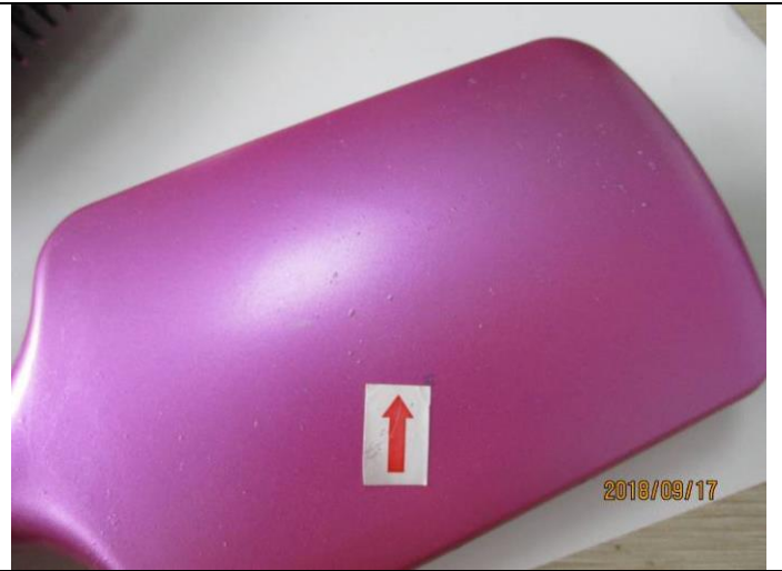
Rough surface – Major
