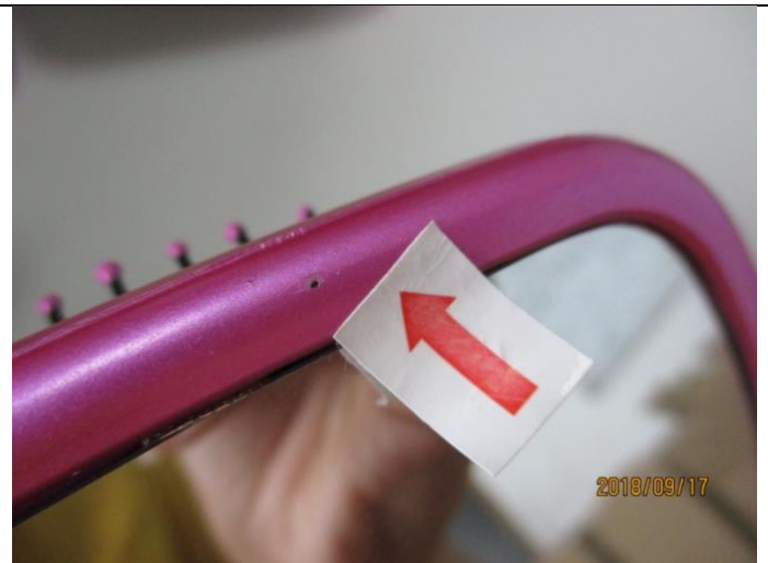
Poor painting – Minor
