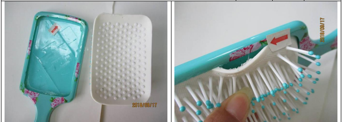
Poor assemble – Major
