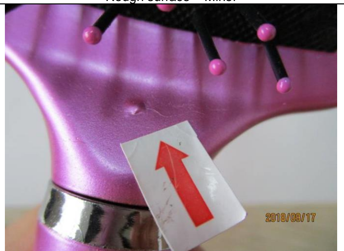
Rough surface – Minor
