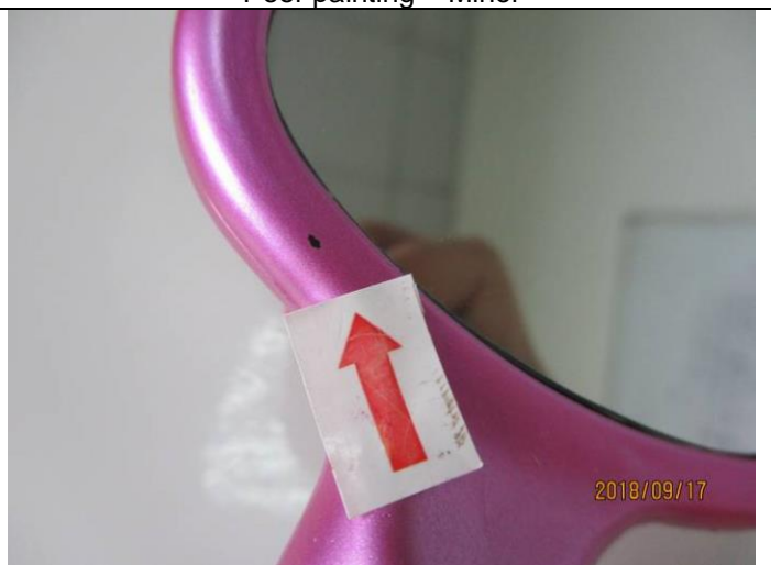
Poor painting – Minor
