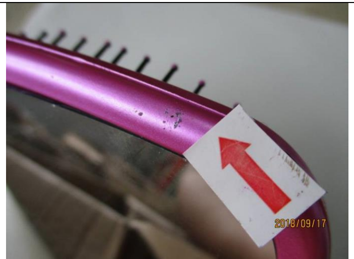
Rough edge /Rough surface – Minor
