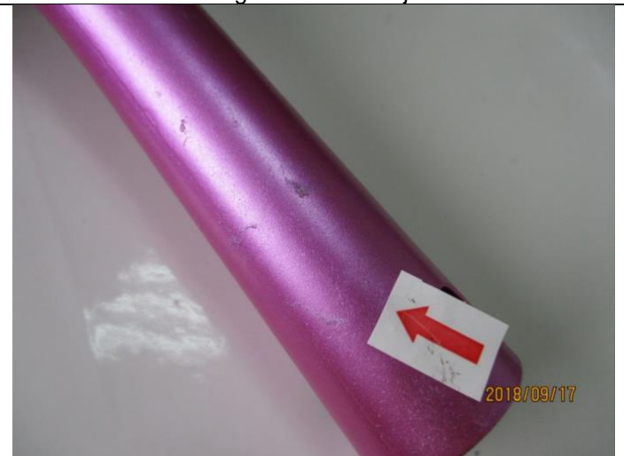
Rough surface – Minor
