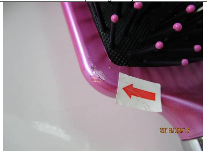
Poor painting – Major
